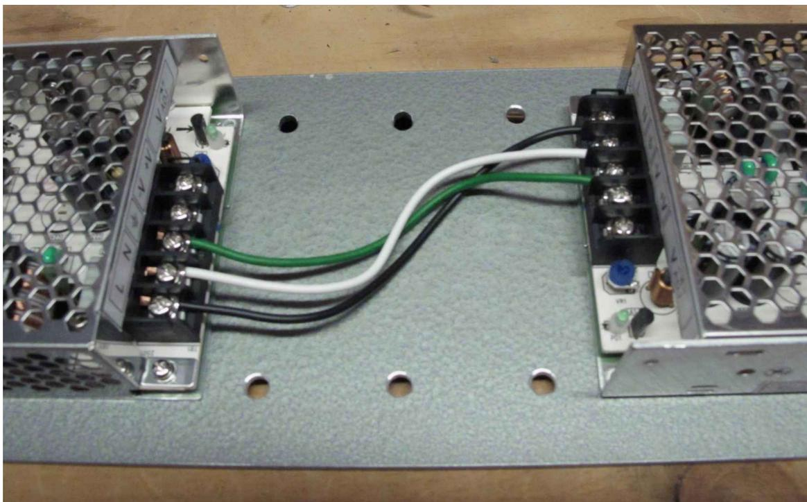
5. Attach the other wires as shown. For now, leave the other end hanging. Tighten the screws.
