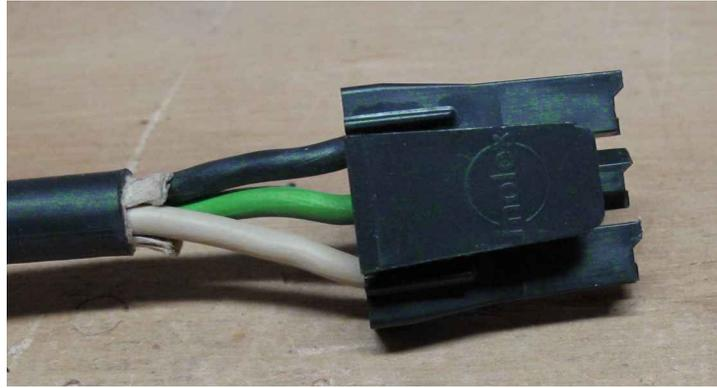
16. Now plug it into the power supply, plug the power supply into AC. Measure the voltage at the console end. It should be 15 volts between adjacent pins, 30 volts from white to black. White is positive.
