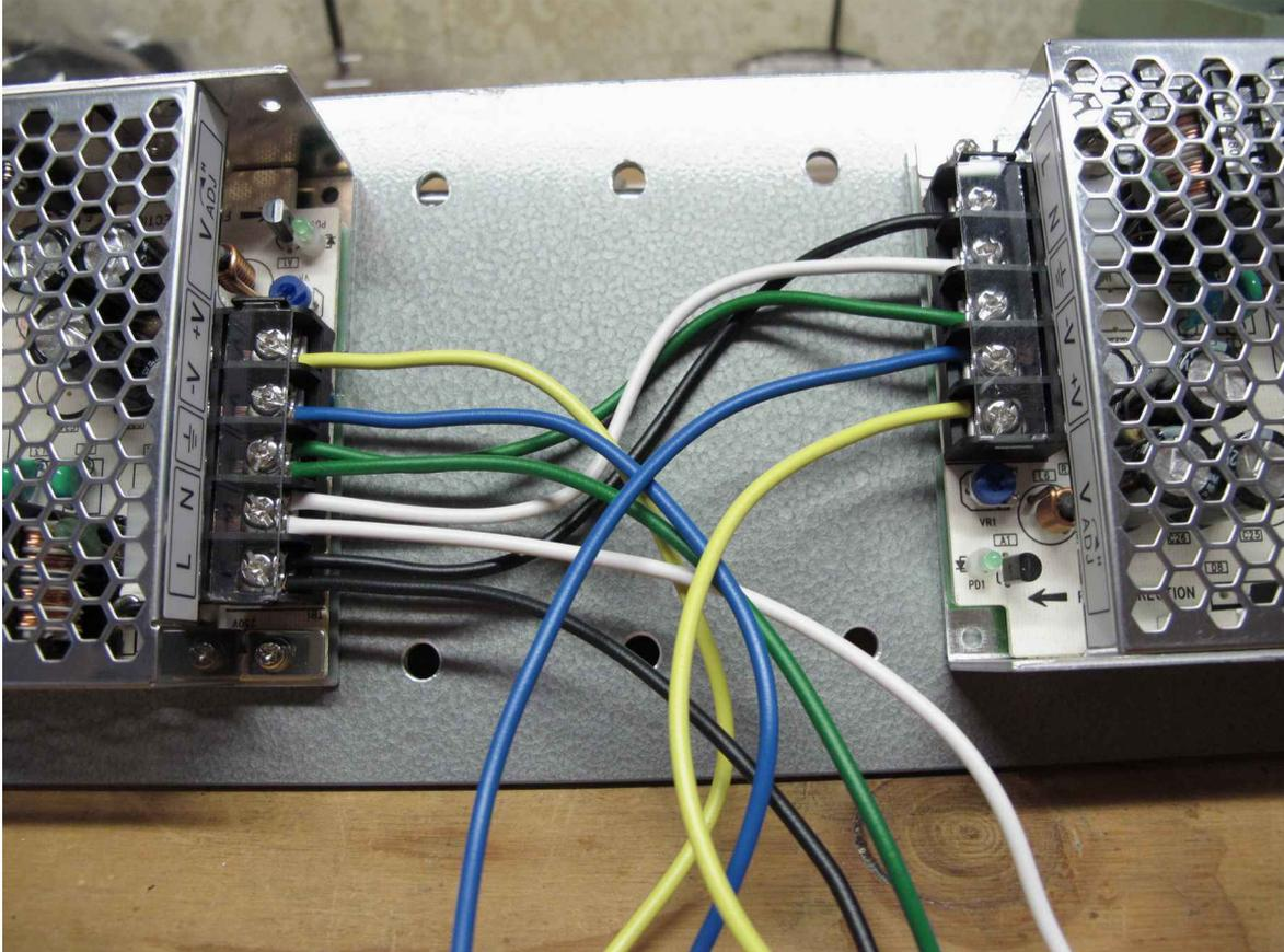
6. Add jumper from ground (green) to -V (blue) on right power supply.
