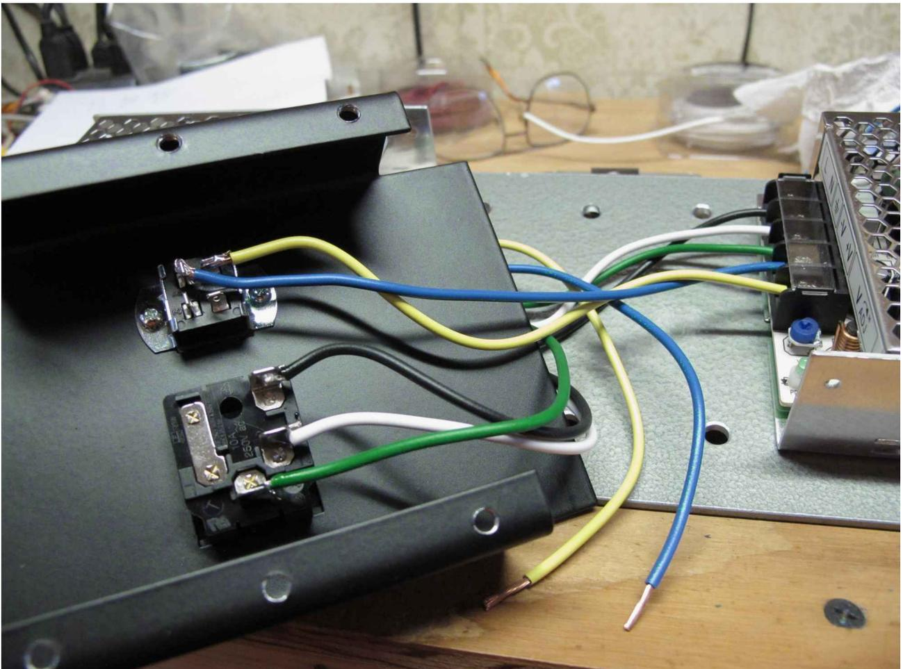
9. Solder the blue and yellow wires from the LEFT power supply to terminals 3 and 4 of the DC “Jones” connector as shown.
