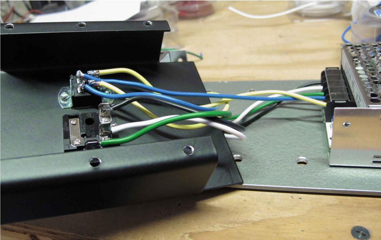
10. Fold the wired cover back and attach with 6 M3 12mm screws. Insert washers between the cover and panel as spacers.
