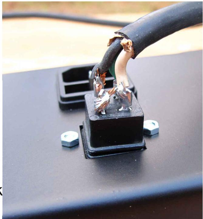
The white wire connects to one plus pin. The black wire connects to the other minus pin. The green wire connects to a plus and a minus diagonally.
