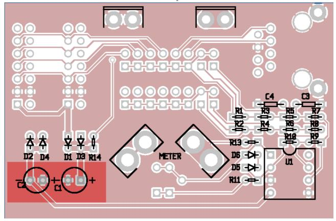
Now insert the IC (LF353, TL072 or equivalent) in the socket U1. Be sure it is in the correct direction.
