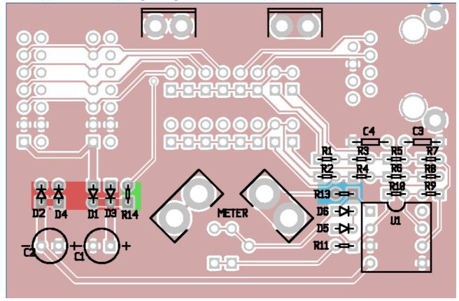
Polarity of resistors doesn't matter electrically, but it is better to be consistent. For stand-up resistors:
